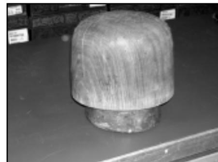
Standard wooden hat block used in manufacturing and repairing hats.
